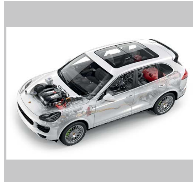
Drivetrain of the Cayenne S E-Hybrid
