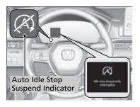
The Auto Idle Stop suspend indicator comes on and a message appears on the gauge when the Auto Idle Stop system cannot be activated.
