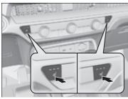
Press the seat heater button: Once - The HI setting (three indicators on) Twice - The MID setting (two indicators on)
