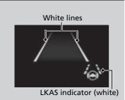
When the LKAS is suspended, green lines on the gauge change to white lines or disappear, and the beeper sounds (if activated).
