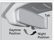
Flip the tab to switch the position.
