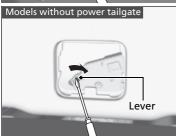
**2.** To open the tailgate, push the tailgate while pushing the lever to the right using a flat-tip screw driver.
